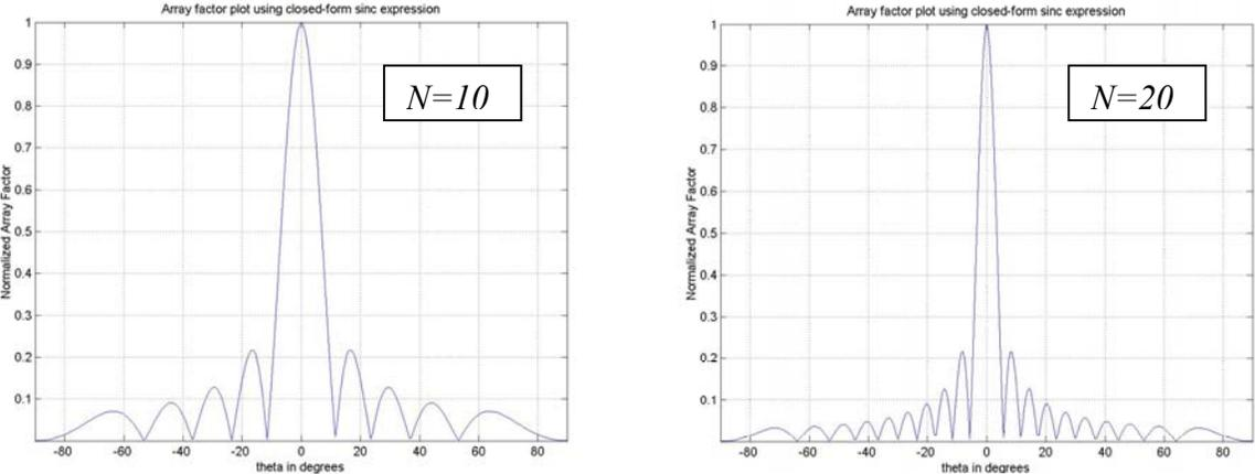
Figure 3.8 Linear plots of the Array factor plots for  $N = 10$  and  $N = 20$  when  $d = \lambda/2$
