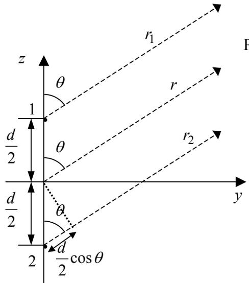
Figure 3.3 Far-field geometry of a two-element linear array
