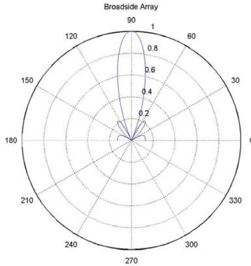
Figure 3.5 Array factor of a 5-element uniform amplitude broadside array
