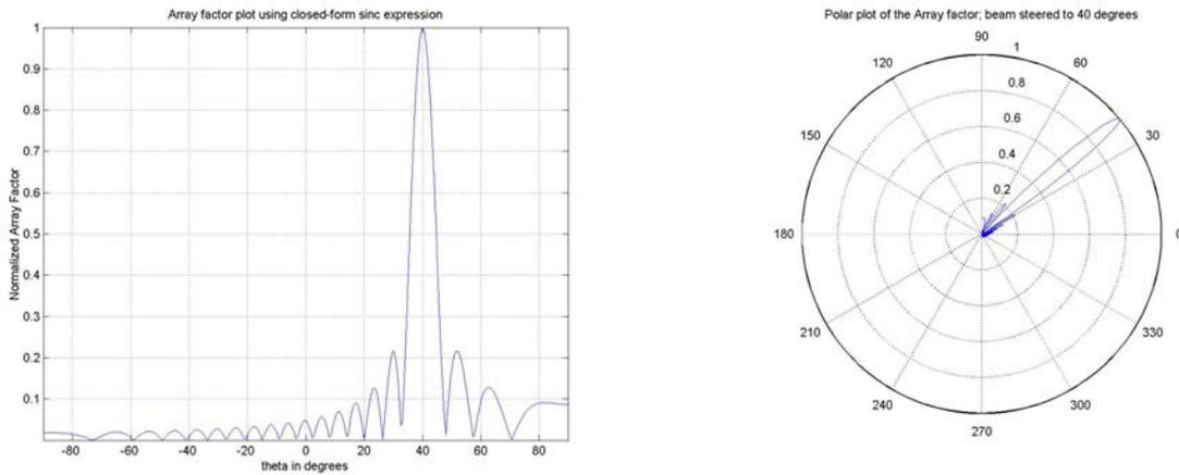
Figure 3.10 Linear and polar plots of the array factor when beam is steered to 40 degrees
