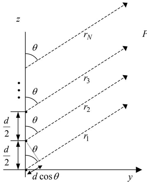
Figure 3.4 Far-field geometry of N-element array of isotropic elements along z-axis
