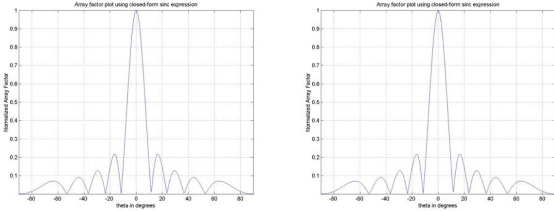
Figure 3.9 Linear plots of the Array factor plots for  $N = 10, d = \lambda/2$  and  $N = 20, d = \lambda/4$
