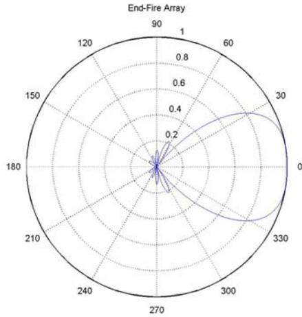
Figure 3.6 Array factor of a 5-element uniform amplitude end-fire array
