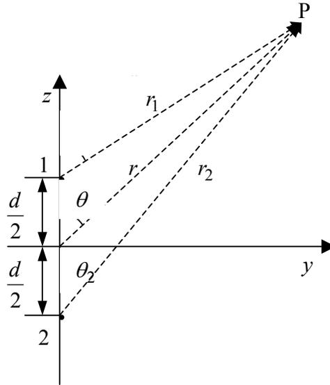
Figure 3.2 A two-element linear array
