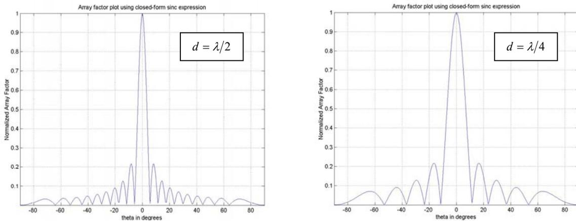
Figure 3.7 Linear plots of the Array factor plots for  $d = \lambda/4$  and  $d = \lambda/2$  when  $N = 20$
