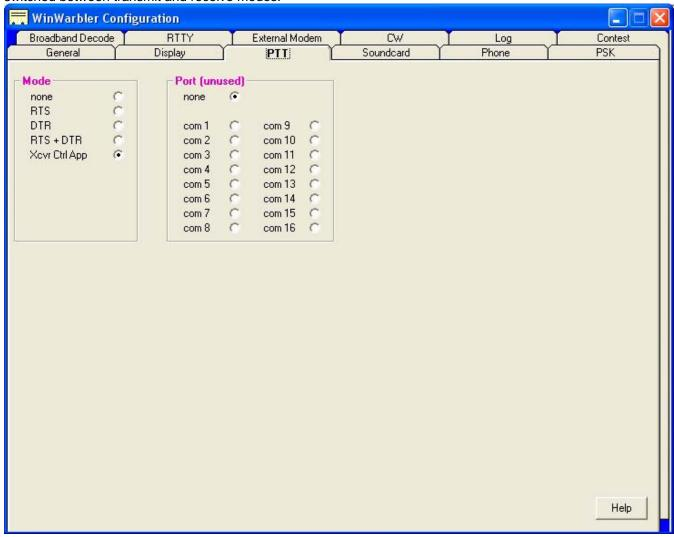
When Soundcard RTTY is active, the specified PTT port is used by the MMTTY engine for PTT (if the PTT Mode is set to RTS+DTR) and/or FSK (if the Soundcard RTTY modulation and transceiver mode panel is set to FSK (USB) or FSK (LSB).
