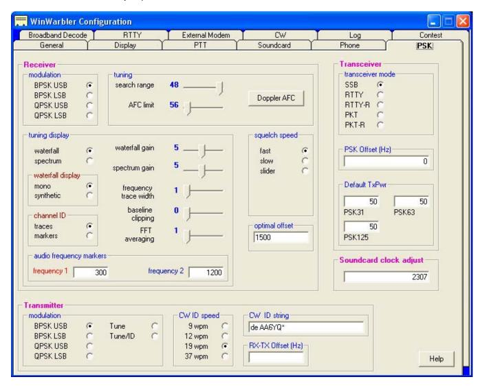
The frequency scale above the tuning display is rendered in green for frequencies within PSK sub-bands, and in red for frequencies outside of PSK sub-bands; you can customize the definition of these sub-bands by copying and editing a file.
