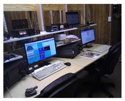
A pair of PW-1 KW auto-tuned amps is shelf-mounted, out of operational view, in the technical workspace behind operating desk. Suspended ceiling "grommets" provide out-of-sight, out-of-the-way, overhead cable-paths for rotor, RX antenna & Stack Match control cables:
